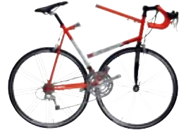
S&S couplings allow you to take your bike in half for easy packing.
